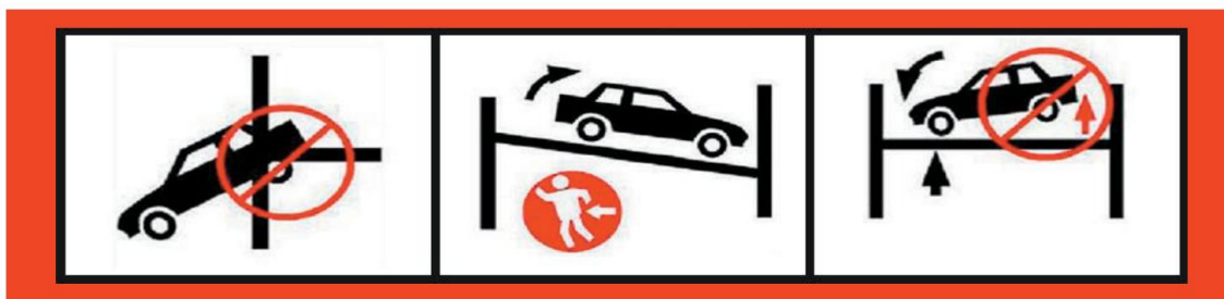
Figure 5.2 — Risk of the vehicle falling from the lift
